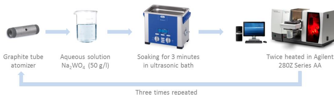
Figure 1 Scheme of graphite furnace surface-modification
