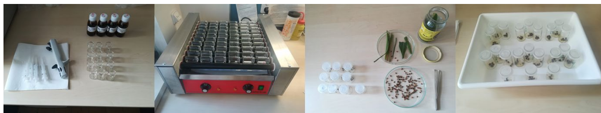
Figure 2 Use of adult-vial-test during testing by IRAC methods
